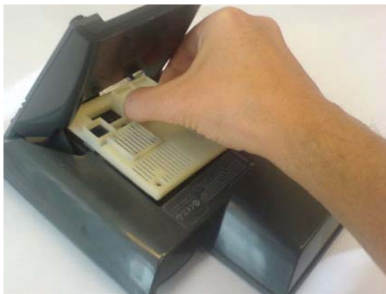
Figure 17: Attaching the option unit
