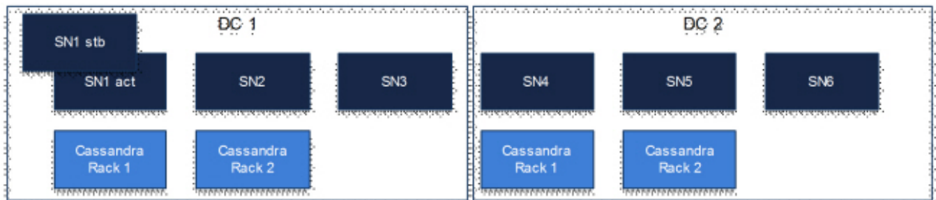
Figure 7: Cassandra with 2 DCs, 4 databases (2 per DC), standalone, i.e. not co-located with SN. 2 racks used per DC. A total of 7 Service Nodes, 6 active plus 1 standby which serves SN1 in DC1.
