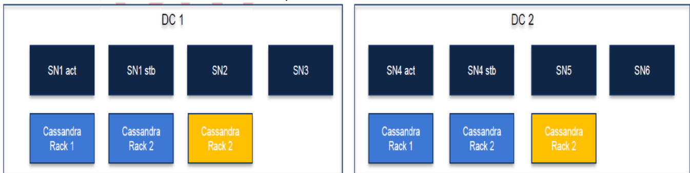
Figure 10: Cassandra with 2 DCs (and 2 clusters), where DC2 is remote, and server redundancy is used in both DCs, i.e. SN1 and SN4 have standby servers.
